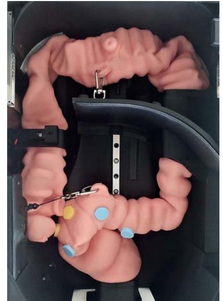
► Fig. 3 External view of the silicon model of the colon. The prototype three-dimensional colon model was prepared using CT images of the human colon. The humanoid-robot simulator has several supporting functions, such as abdominal compression and repositioning of the diaphragm as if through deep inspiration.
