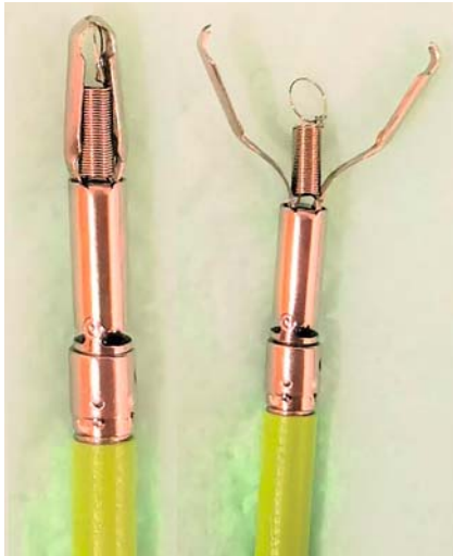
► Fig. 1 Photograph of the novel clip-with-spring device, which consists of a metal clip and a spring fixed between the two claws.
