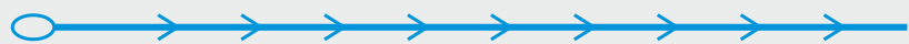
► Fig. 2 Schematic showing the barbed string. The barbs were unidirectional, which enabled tight stretching. There were 8 barbs per centimeter of string, at an angle of about 15° to the thread.
