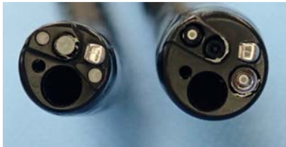
► Fig. 1 Comparison of the novel therapeutic thin endoscope and normal diameter therapeutic endoscope. Left: Novel therapeutic thin endoscope has a 7.9-mm outer diameter and 3.2-mm working channel diameter. Right: Normal diameter therapeutic endoscope with a 9.8-mm outer diameter.
