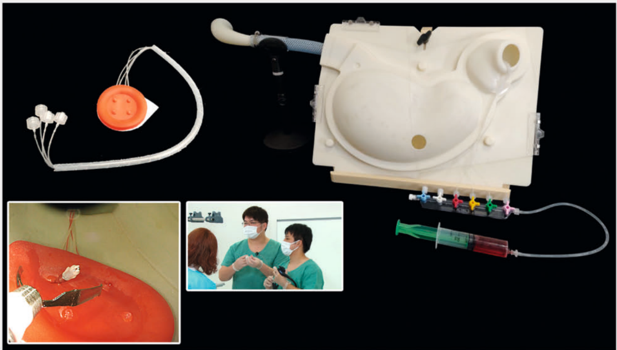
► Fig. 2 The appearance of the simulator model. The ulcer model can reproduce pulsatile bleeding from selected vessels that can be affixed anywhere in the stomach and duodenal lumen (upper left). Endoscopic image of simulated bleeding (bottom left). The lumen model from the pharynx to the duodenal portion: simplified from human 3D data and waterproof and impact-resistant (right).
