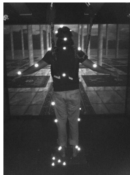
Fig. 1 Marker placement and experimental set-up.
