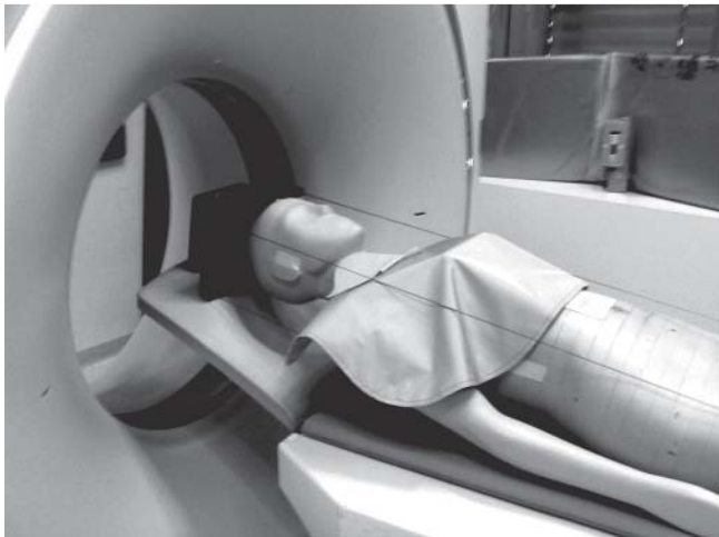
Fig. 2 MAVIG RP648 cover for thyroid, sternum, chest and shoulder area with 0.35 mm lead equivalent inlay placed on the CIRS ATOM anthropomorphic female adult phantom Irene.
