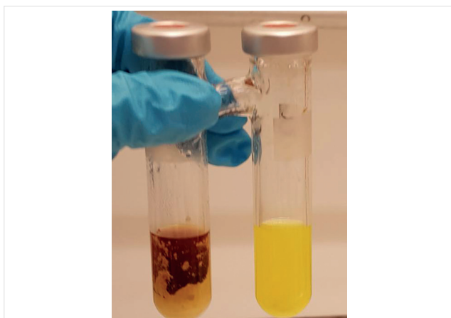
Figure 2 Two-Chamber vial after radical carbonylation reaction. Left-hand chamber ( C_{CO} ) contains DBU/Mo(CO) 6 , right-hand chamber ( C_{rxn} ) contains reactants. 34
