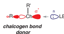
Figure 1 Chalcogen bonding as n \rightarrow \sigma^* type interaction between a Lewis base (LB) and a chalcogen bond donor (Ch = S, Se, Te)
