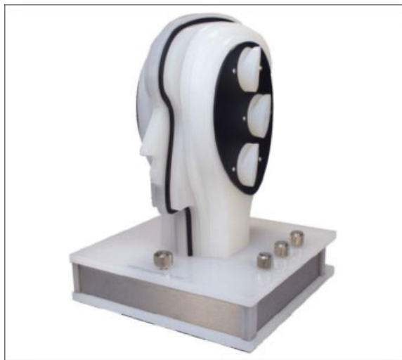
Figure 2 Klangfinder acoustic manikin head. Three ear simulators are mounted on either side of the head to obtain measurements from three pairs of hearing aids at the same time.
