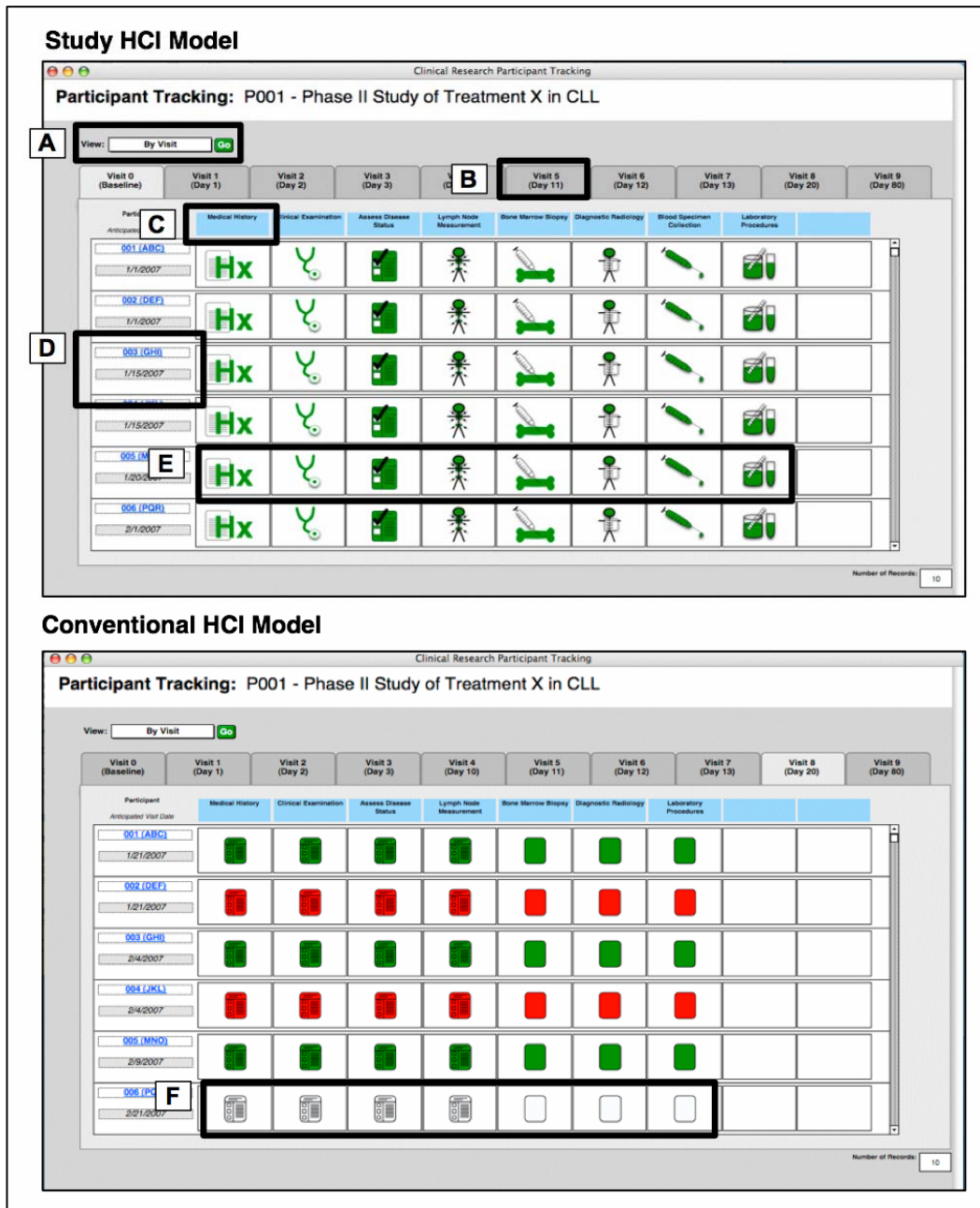
Fig. 4 Illustrative example of prototype CTPT HCI models. Notable features include: A) the ability to filter the end-user view of records by visit, protocol or participant; B) a tabbed interface model for navigating between visit days as defined by the study protocol; C) optional textual labels to accompany icons; D) result-set rows corresponding to a specific trial participant; E) prototype icons designed using PD which indicated from left-to-right: medical history, physical exam, case report form, lymph node measurement, bone marrow biopsy, radiology, blood specimen collection and laboratory procedures; and F) conventional icons adapted from commonly available CTPT software.
