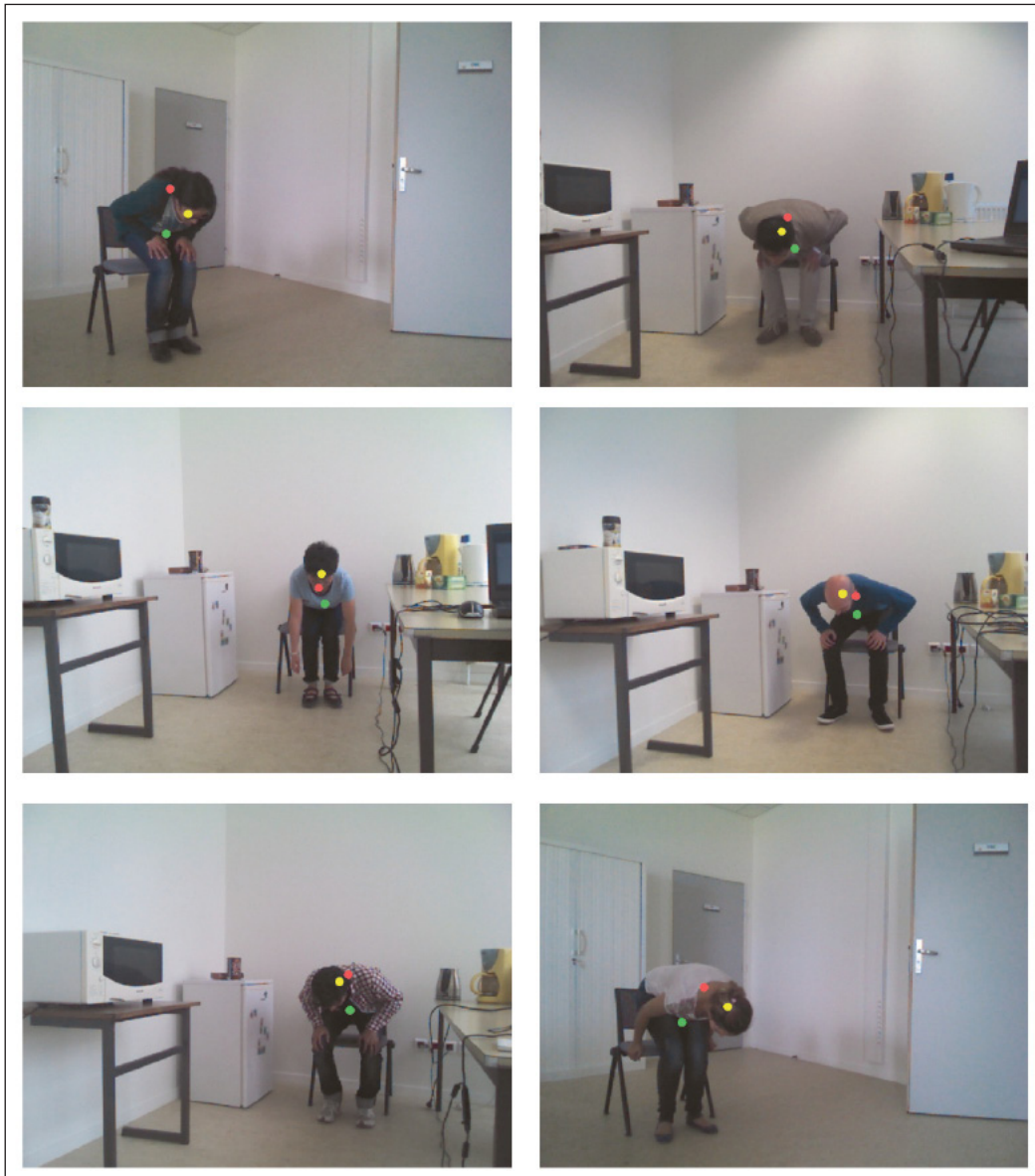
Fig. 8 Detection of the shoulder center (green circle), the head center (yellow circle) and the center of mass (pink circle); and comparison between the angle \alpha_1 calculated according to the Kinect skeleton and \alpha_2 calculated according to 3D extracted points using the proposed method. (a) \alpha_1=47.47^\circ ; \alpha_2=71.02^\circ . (b) \alpha_1=16.77^\circ ; \alpha_2=99.53^\circ . (c) \alpha_1=28.31^\circ ; \alpha_2=82.02^\circ . (d) \alpha_1=51.47^\circ ; \alpha_2=84.80^\circ . (e) \alpha_1=51.64^\circ ; \alpha_2=84.61^\circ . (f) \alpha_1=49.67^\circ ; \alpha_2=104.63^\circ .
