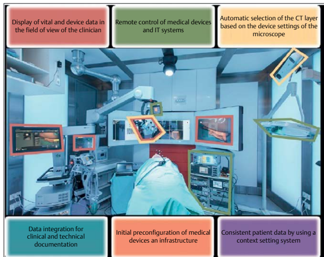
► Fig. 18 Ergonomic experimental setup of the technical components of the OR.NET in the ICCAS for ENT-surgical applications (figure taken from ICCAS Leipzig [3, 80]).
