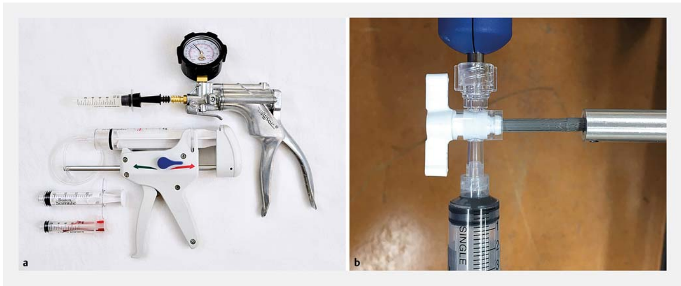
► Fig. 1 a Aspiration devices pictured left to right: 10-cc EUS-FNA syringe (B. Braun Medical Inc.), 20-cc EUS-FNA syringe (Boston Scientific), 50-cc Alliance II Syringe System (Boston Scientific), and a nonmedical hand vacuum pump connected to a syringe barrel via rubber adapter. b Application of high-frequency oscillation to the needle syringe interface in FNA using a Honda transducer.
