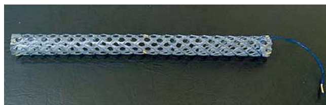
► Fig. 1 The FCSEMS-MH (M.I.Tech Co., Ltd, Pyeongtaek, Korea) has non-flared ends, a silicone covering membrane and a long lasso to facilitate stent retrieval. The stent has a unique design featuring 2.5-mm holes located in the center of the membrane of each cavity, which prevent bile duct side branch obstruction and stent migration.
