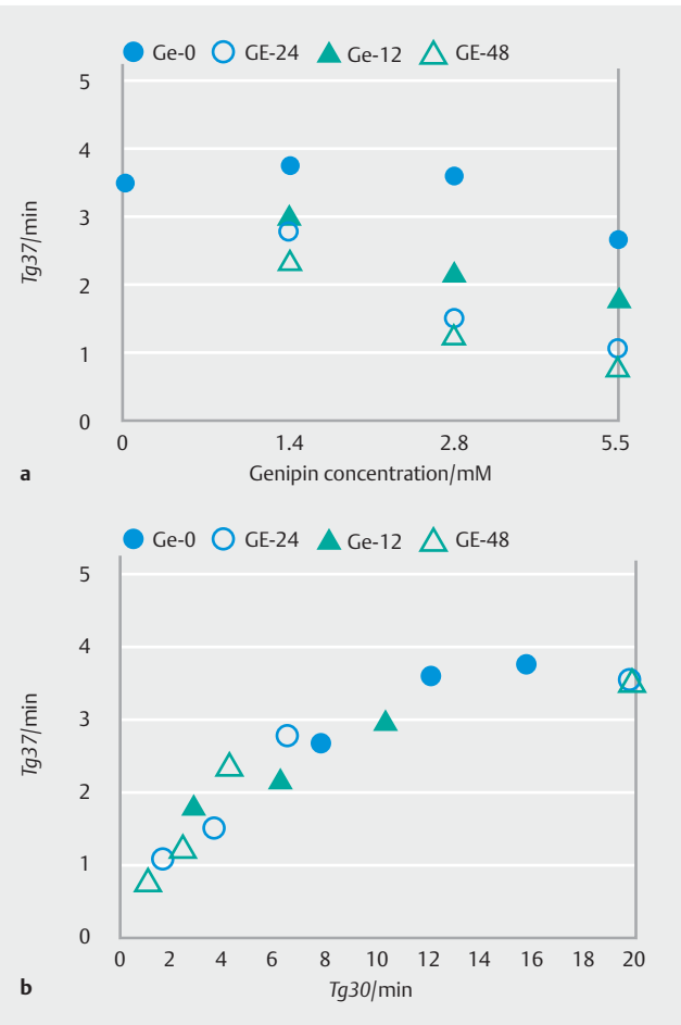
► Fig. 2 a Effects of genipin concentrations on Tg_{37} of the PSC/Ge sols containing various Ge samples. b Plots of Tg_{37} against Tg_{30} of the PSC/Ge sols containing various Ge samples at concentrations 0–5.5 mM.
