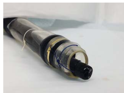
► Fig. 3 The endoscope was fixed 2 mm from the distal tip of the overtube and connected to the overtube at four points using silk thread.
