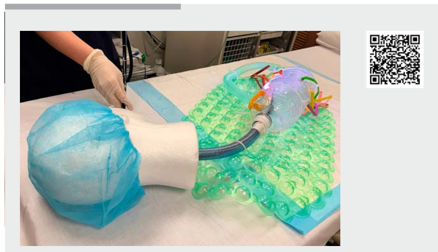
► Video 1 A low-cost endoscopy training model for novice endoscopy training.
