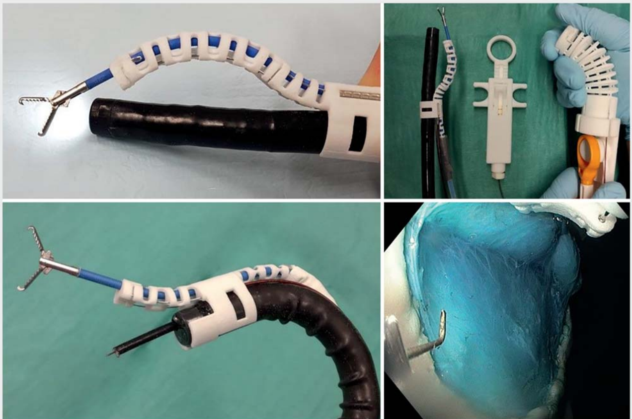
▶ Fig. 3 Behind-the-tip mounted and tip-mounted single-arm manipulators.
