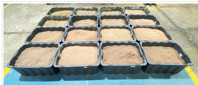
Figure 10 A mercury sorbent made from canola oil and sulfur can be manufactured on a multi-tonne scale. A 500 kg sample manufactured by Clean Earth Technologies is shown in the image. Reprinted with permission from Clean Earth Technologies.
