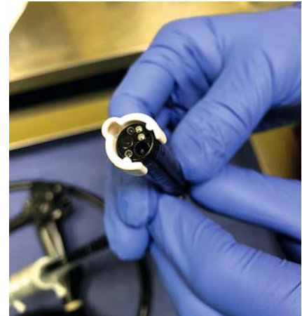
► Fig. 3 Closer view of the additional working channel on the tip of the scope.
