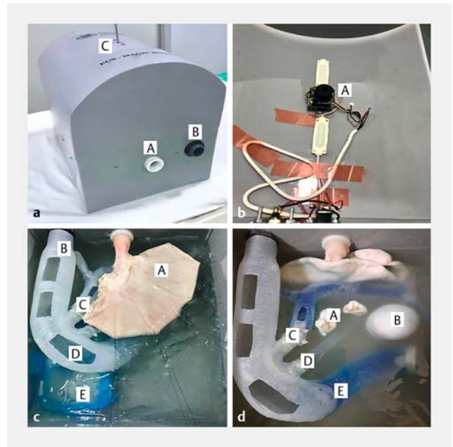
► Fig. 1 a EUS Magic box exterior. Note two separate opening for (A) stomach and (B) duodenum and (C) external control for camera on the roof. b The inner view of the roof showing the internal camera (A) with light. c The interior of the model after removing the roof. The pig stomach (A) is sutured to the side of the box with thread. The ultrasound gel medium bathes the organs. The duodenum (B) is attached to a separate inlet, and has holes (D) to see guide wire movement, when X-ray is not being used. The bile duct (C) and pancreatic duct are underneath the pig stomach, and can be seen converging toward the papilla. The electrocautery pad is seen submerged in the gel medium (E). d Interior of model after pulling the stomach away. Note pig liver tissue (A) for biopsy and pancreatic pseudocyst (B) made up of pig urinary bladder. The dilated bile duct (C) and pancreatic duct (D), can be seen joining at the papilla. The third part of the duodenum is submerged in the medium. It can be filled with water, and used as enteral loop (E) for EUS-GE.
