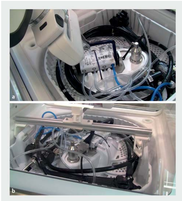
► Fig. 3 Preparatory steps for the removal of the adapted tray with the processed endoscope from the EWD. a Lifting of the lever to separate the individually connected lines b removal of the tray with the special lifting device.
