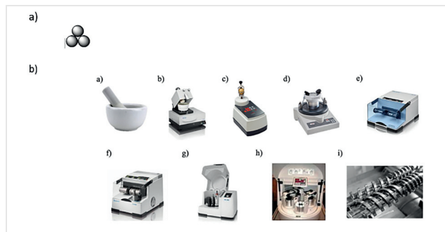
Figure 1 (a) Representation of mechanochemical activation advanced by Hanusa. (b) Typical grinding and milling equipment. (a) Mortar and pestle. (b) Retsch automated mortar. (c) Fritsch vertical shaker mill. (d) Fritsch vibrational mill. (e) Retsch vibrational ball mill. (f) Retsch vibrational ball mill with controlled temperature (Cryomill). (g) Retsch planetary ball mill. (h) Multiple-sample mill (Automaxion). (i) Twin-screw used for continuous mechanochemical extrusion. Reproduced with permission from ref 2e. Copyright 2020 The American Chemical Society.
