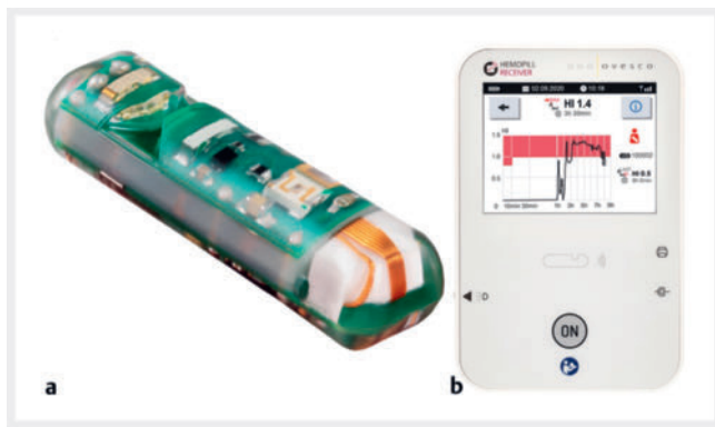
► Fig. 1 a The swallowable bleeding sensor capsule, HemoPill, measures 26.3 mm x 7 mm with a measuring gap for photometric measurements. b Proprietary HemoPill receiver, which plots the photometric measurement results over time. This figure displays an example of a positive blood detection, showed by a HI within the red zone. Source: Ovesco Endoscopy AG, Tübingen, Germany
