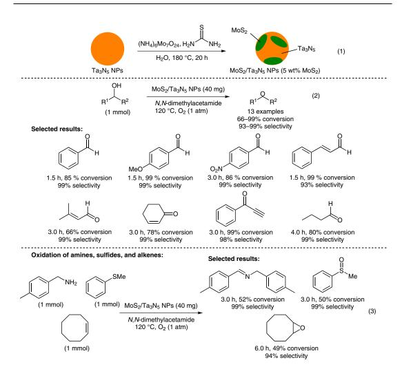
**Significance:**  $Ta_3N_5$  nanoparticles partly coated with a  $MoS_2$  layer ( $MoS_2/Ta_3N_5$  NPs) were prepared by hydrothermal treatment of  $Ta_3N_5$  NPs with ( $NH_4$ ) $_6Mo_7O_{24}$  in the presence of thiourea (eq. 1).  $MoS_2/Ta_3N_5$  NPs catalyzed the aerobic oxidation of alcohols under oxygen (1 atm) to give the corresponding aldehydes or ketones in up to 99% conversion with 99% selectivity (13 examples, eq. 2).
