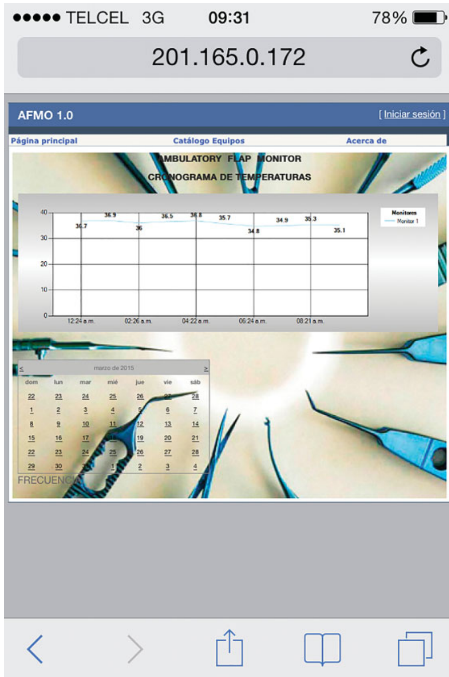
Fig. 2 Screen shot of a mobile phone with the web application running. We can see the temperature graph in real time.
