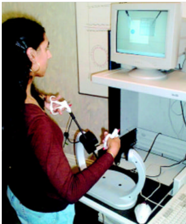
Fig. 1. Minimally Invasive Surgery Training-Virtual Reality (MIST-VR) trainer (Mentice Medical Simulation AB, Gothenburg, Sweden).
