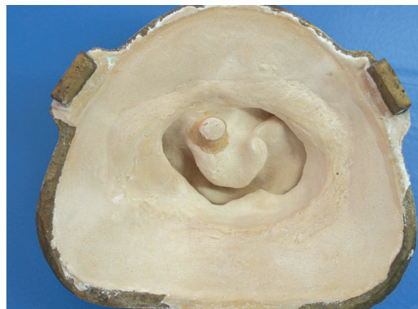
Figure 4. Completed mold with space created by the wax pattern.
