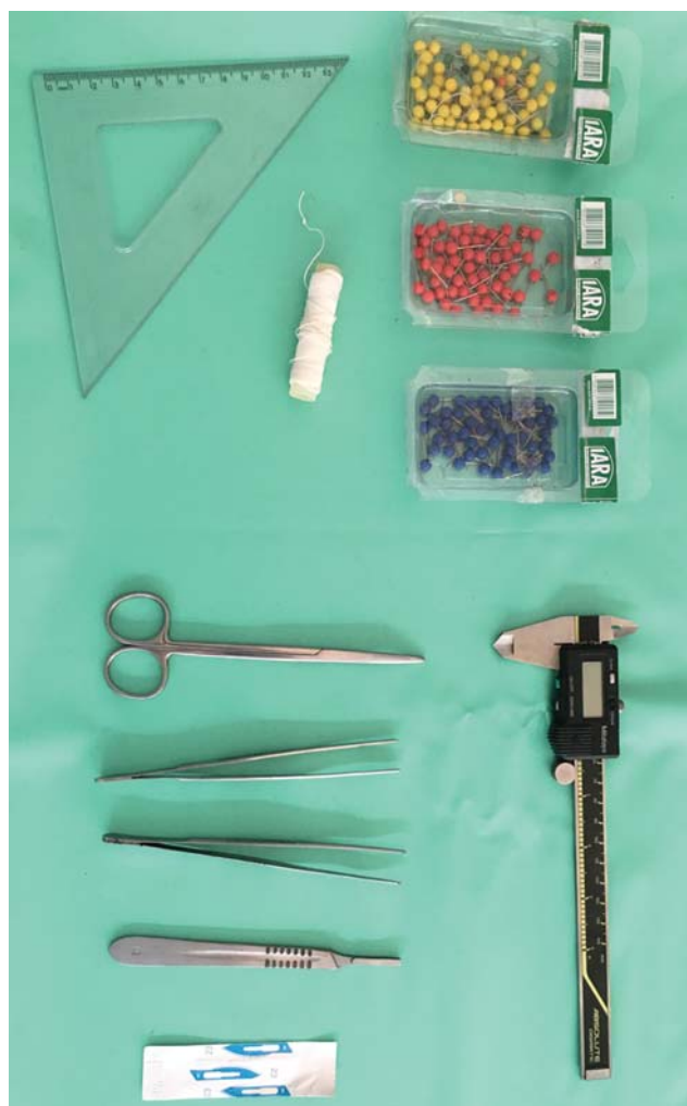
Fig. 1 Material used for the dissection: scalpels with number 3 and 4 handles, Metzenbaum scissors, anatomical and toothed clamp tweezers, and Digimess digital caliper.
