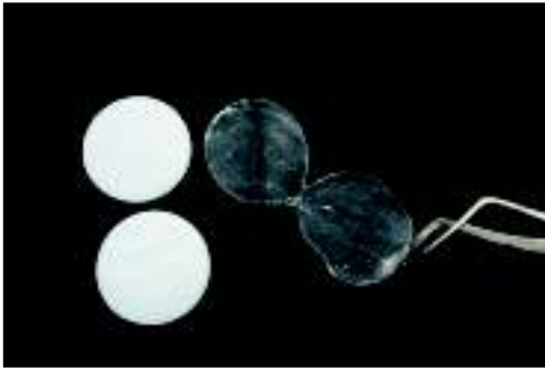
Matrix button, before and after softening
