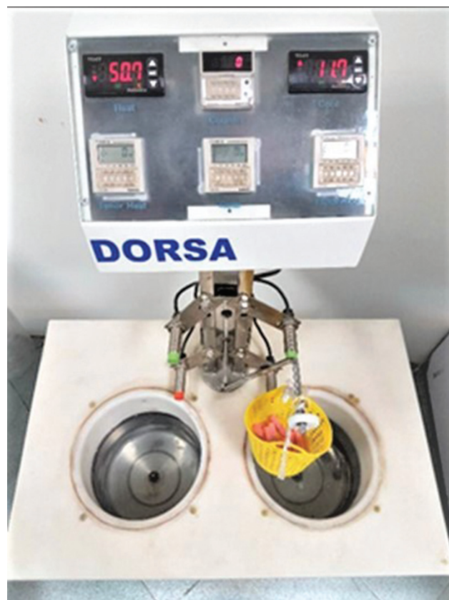
Fig. 4 Thermocycling machine (3000 thermal cycles in 5 and 55°C temperatures with a dwell time of 30 seconds).
