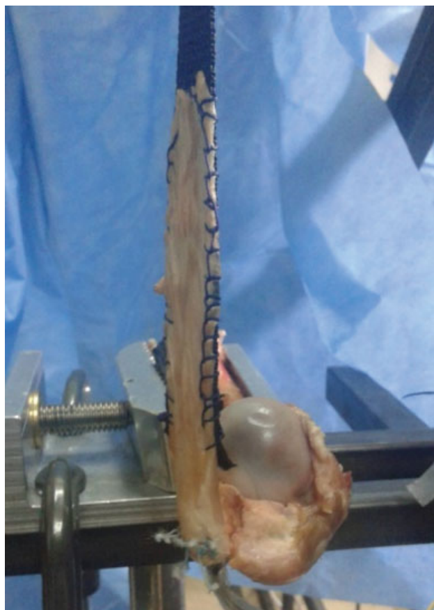
Fig. 3 Modular support. The modular support was adjusted to ensure that the tendon was parallel to a vertical line.
