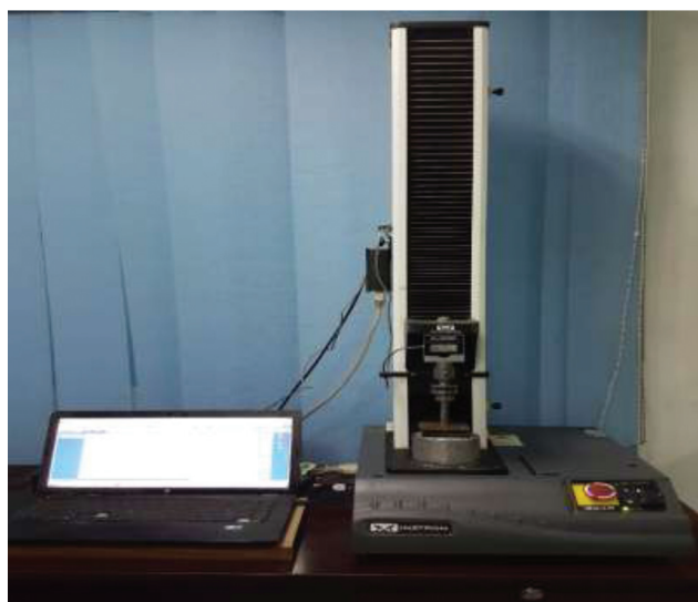
Fig. 2 Push-out testing machine (Instron Industrial Products, Model 3345; Massachusetts, United States).
