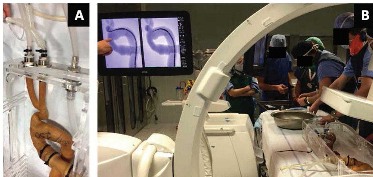
Fig. 2 Silicone three-dimensional (3D) printed model, used to perform a simulation before a real surgical procedure in a patient suffering from an aortic arch aneurysm. (A) The 3D model is connected to a pulsatile flow system to simulate the antegrade flow. (B) Surgical simulation phase in the operation room.
