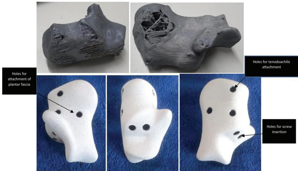
Fig. 3 Prototype of the implant and custom-made final prosthesis coated with hydroxyapatite.
