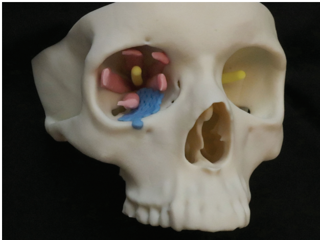
Fig. 11 Material jetting. Patient presented with a malpositioned, right orbital floor implant. A material jetting printer (J5, Stratasys, Eden Prairie, MN) was used to generate a model of the defect and surrounding anatomy. The tactile model illustrated the plate's (blue) proximity to her optic nerve (yellow) and extraocular muscles (pink). Utilizing the model, the clinician was able to further develop a surgical plan and successfully illustrate the risks and benefits of removing the malpositioned implant to the patient.
