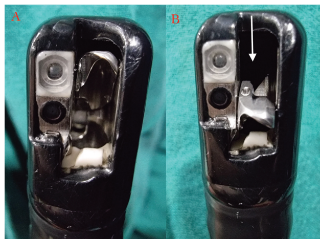
Fig. 1 Sideview duodenoscope with elevator channel in open (A) and closed position (B), with recess under the elevator channel (arrow).
