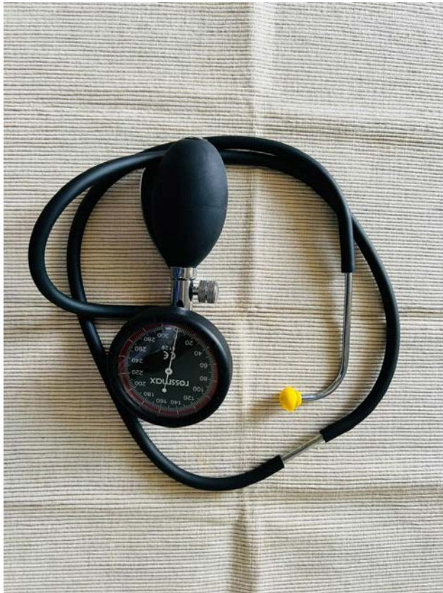
Fig. 1 Prototype of the Eustachian barotubometer designed by the first author.
