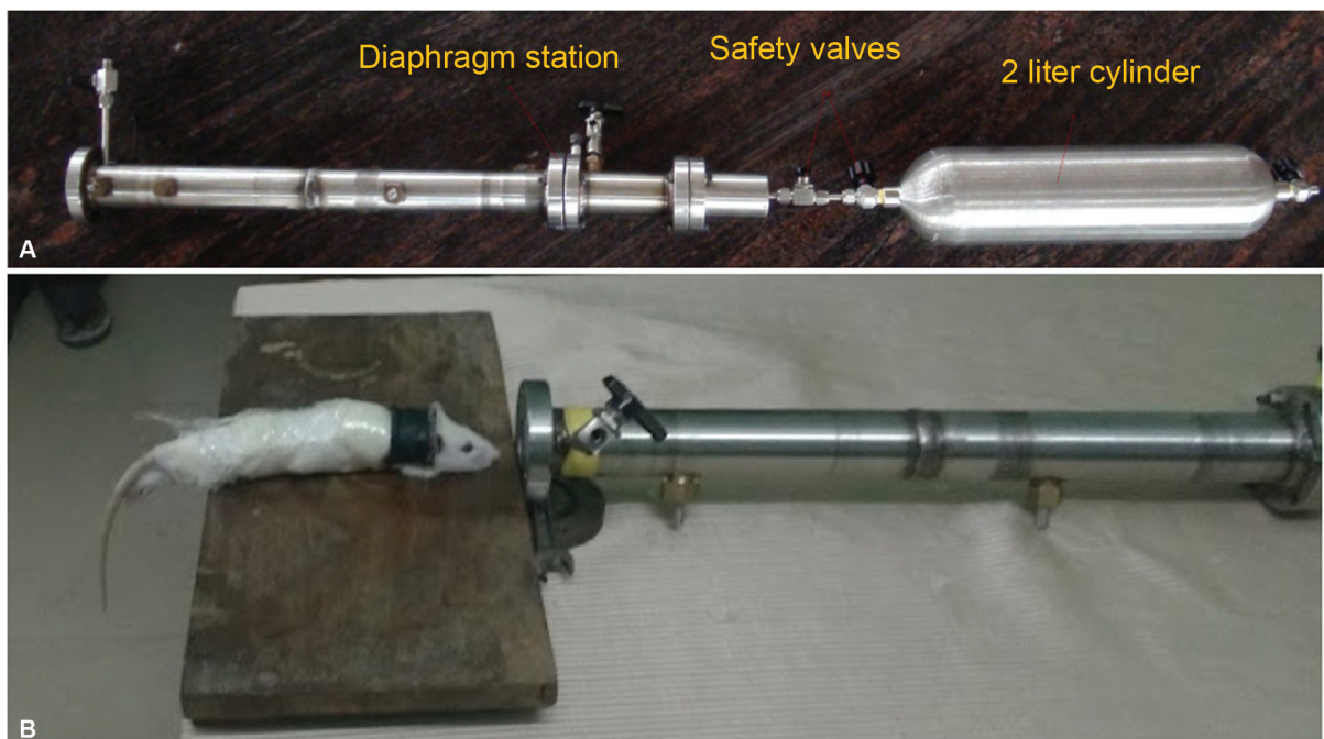
Fig. 1 (A) Modified Reddy's gas-driven shockwave tube. (B) Rat restrained in front of the open end of the modified Reddy's tube.
