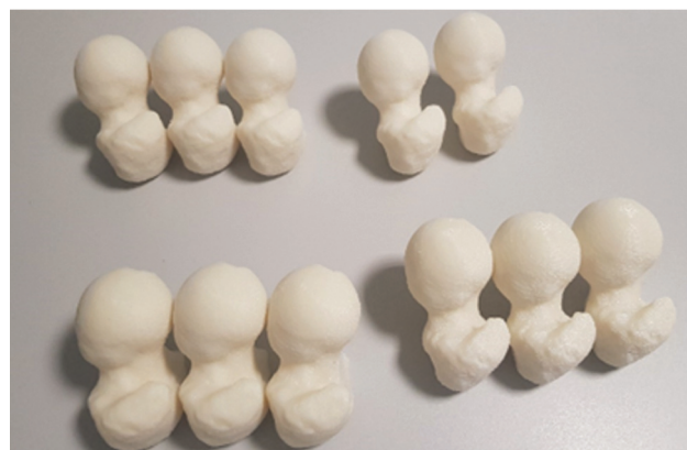
Fig. 2 Femurs with deformities printed on ABS plastic. Source: Author, December 2022.
