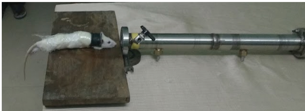
Fig. 1 Rat restrained in front of the open end of the modified Reddy's tube.
