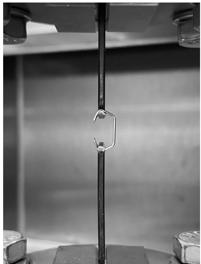
Fig. 1 Photograph of a fired stapler attached to the materials testing machine for evaluation. The upper and lower hooks of the machine are mounted at the level of the limbs of the staple. The first flexural deformation that occurred was recorded as a failure.
