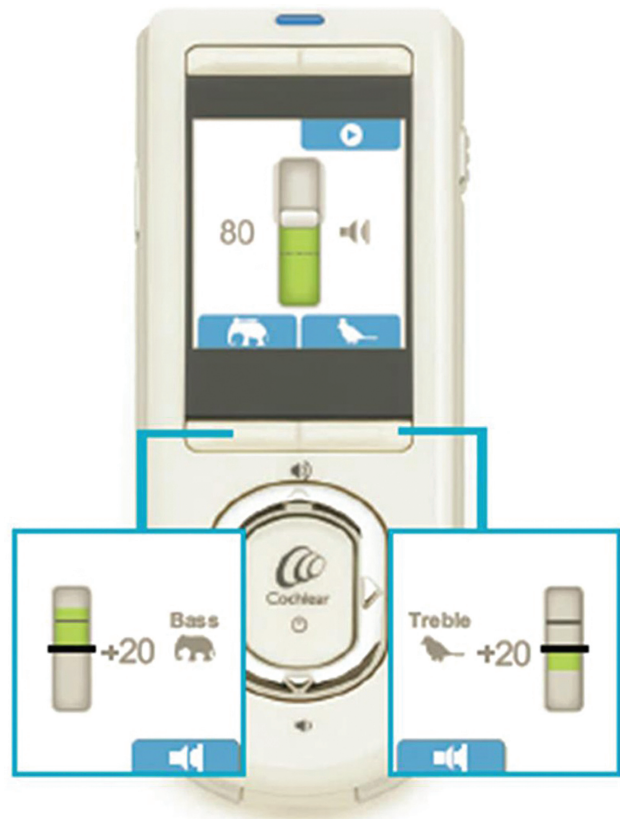
Fig. 2 The CR110 remote assistant with the modification functions in master volume (central screen), bass, and treble (smaller frames on the left and right, respectively). 17
