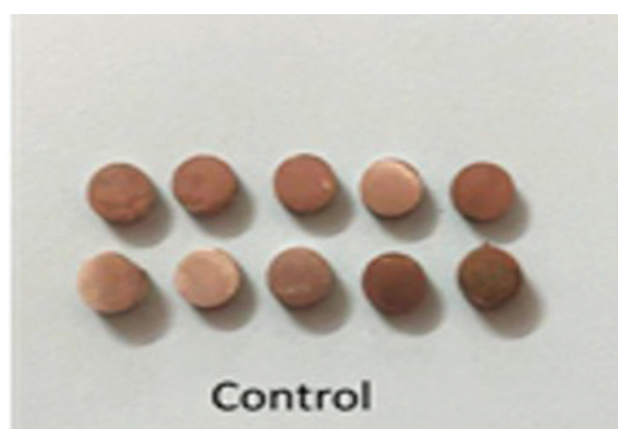
Fig. 2 Samples for electrophoretic deposition (EPD), titanium 6 aluminum 4 vanadium (Ti-6Al-4V) substrate (20 × 10 × 2 mm).
