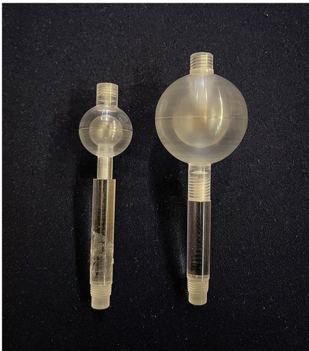
Fig. 1 Double-sphere phantom. The inner/outer diameters of the spheres were 13/22 mm (left) and 22/37 mm (right).
