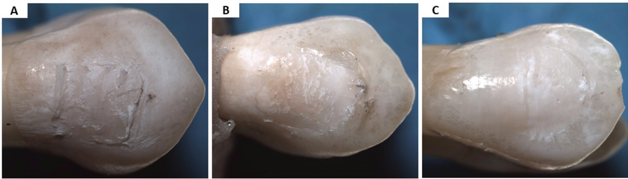
Fig. 1 ARI scores for different groups. (A) Remnant adhesive represents score 2; (B) remnant adhesive represents score 1; (C) ARI score 0. ARI, adhesive remnant index.
