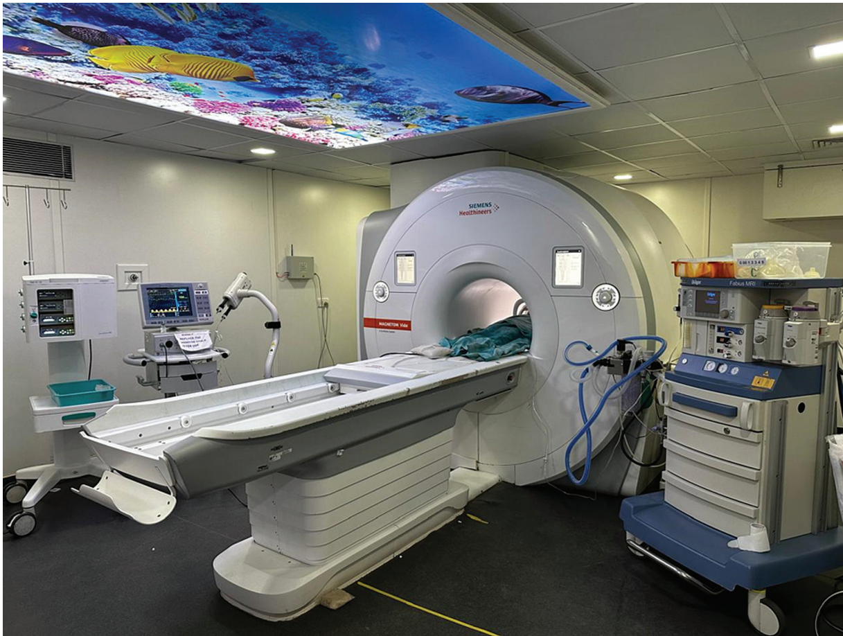
Fig. 4 Positron emission tomography magnetic resonance imaging (PET/MRI) room setup showing the patient gantry, anesthesia machine, monitor, and infusion pumps.
