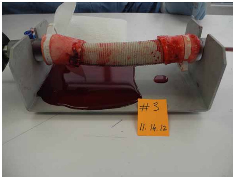
Figure 8. This picture is from experiment 3; this time, the stapled side is on the right and the hand-sewn on the left. The pressure inside the aorta-graft was increased to 80 mm Hg, and there was a large pool of bovine blood on the hand-sewn side. There was very little leakage from the stapled side even at this pressure.
