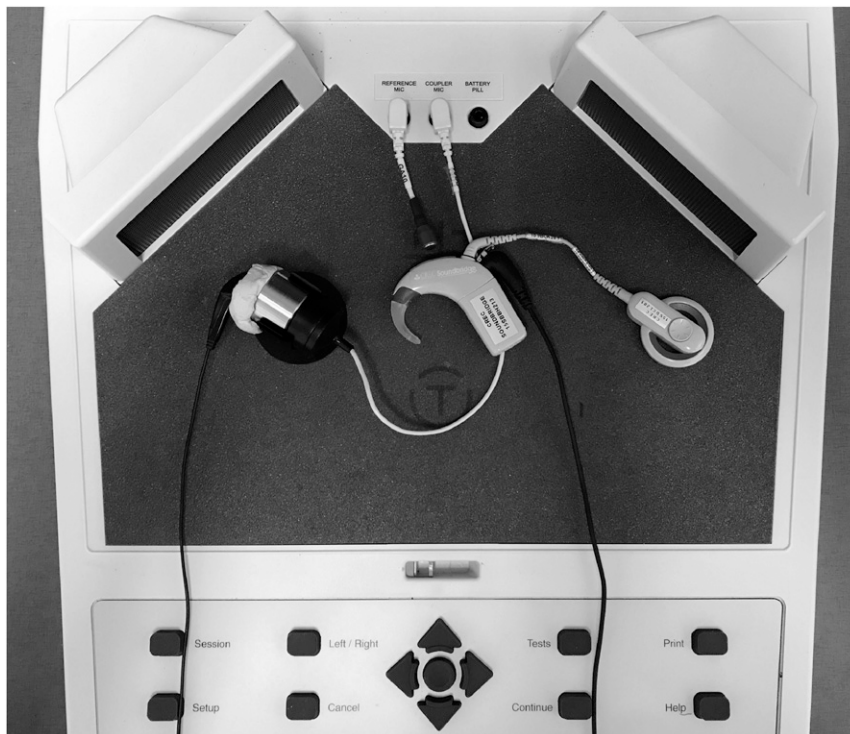
Figure 1. Configuration for Step 1 for a Cochlear N6 sound processor coupled to a MM2+ with and without a Phonak Roger DM system. The Cochlear N6 sound processor is in the Verifit chamber.
