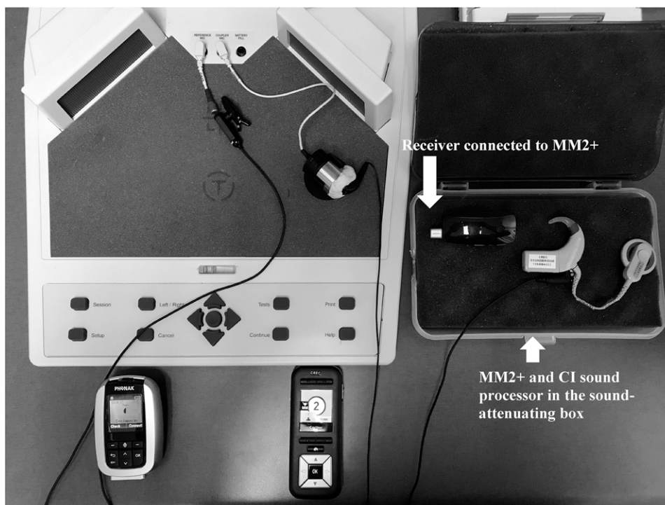
Figure 4. Configuration for Step 2 for a Cochlear N6 sound processor coupled to a MM2+ and a Phonak Roger DM system. The Phonak Roger transmitter microphone is in the Verifit chamber. The MM2+ and the Cochlear N6 sound processor are in the sound-attenuating box.
